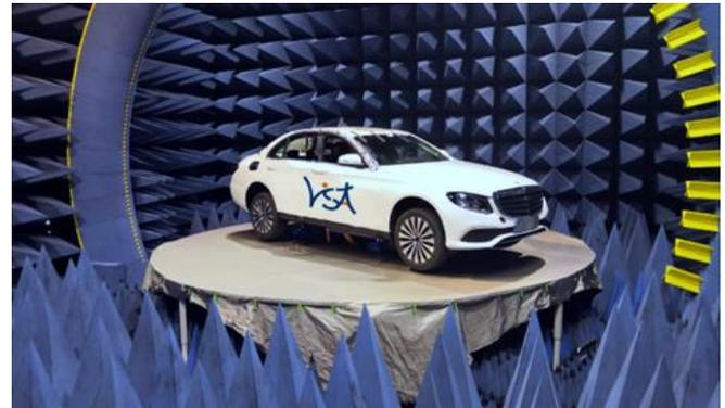
Shielded anechoic chamber (VISTA)
